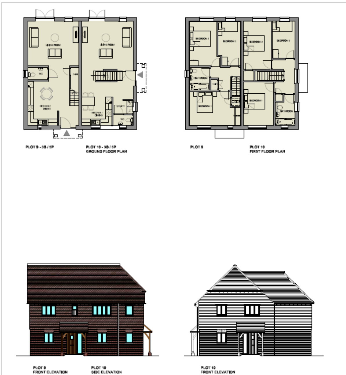
Figure 4: Corner turning 3-bed semi-detached units
